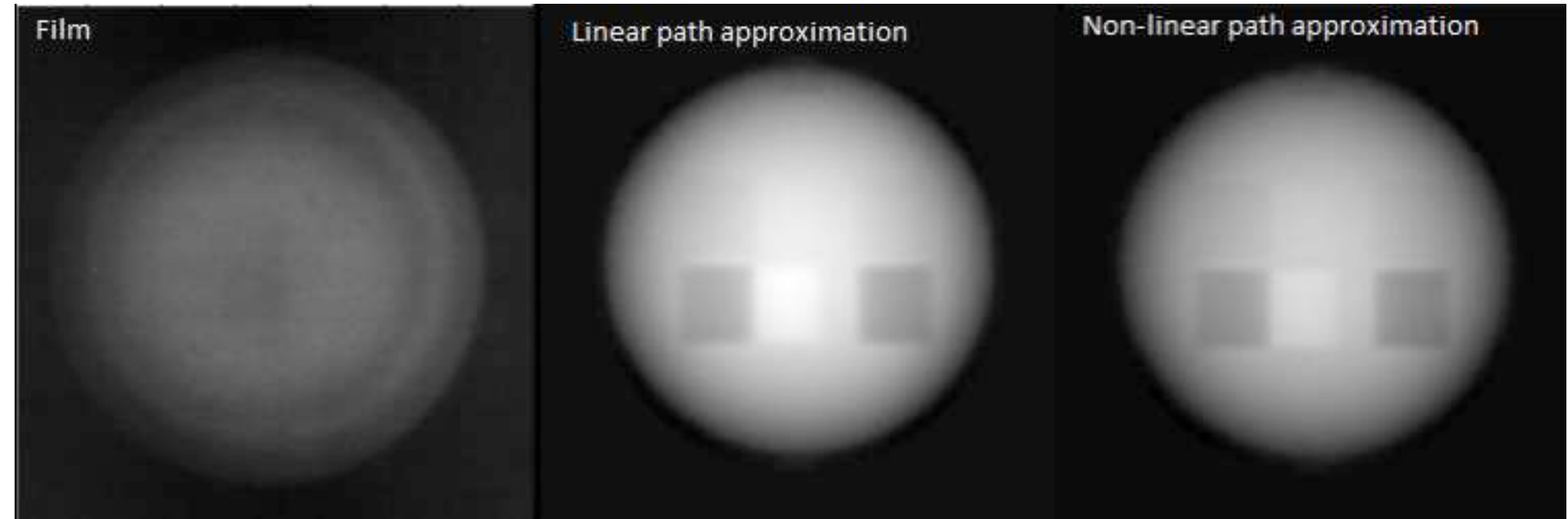
Comparison of film radiograph and radiographs from the PRaVDA system
