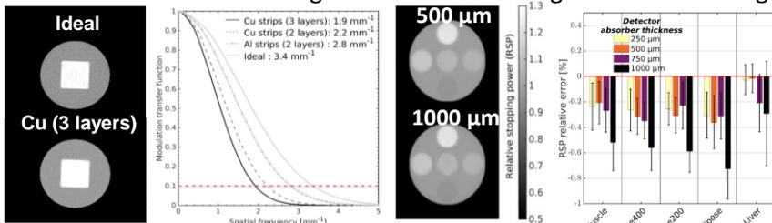
**Final choice of tracker with Al strips and range telescope with 600  $\mu\text{m}$  mylar plates**
