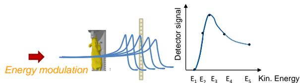
Large area **CMOS detectors** with linear signal decomposition method to determine WET
