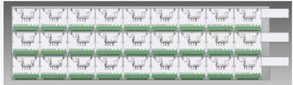
Flexible carrier board modules (3 x 9 chips)
